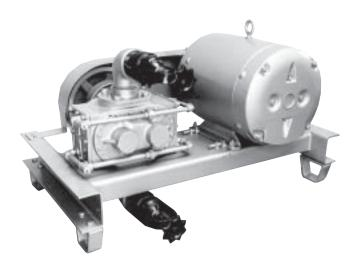
**Skid Mounted** with Etnyre P-200 steam/hot oil jacketed bituminous pump with relief valve. 15HP 1200 RPM 230/460 volt, 3 phase 60 cycle Electric Motor, four V-belt drive, heavy duty steel frame, 3" piping with two Etnyre quick couplers. Weight, 900 lbs. uncrated.
