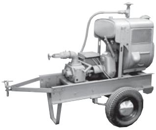
**Trailer Mounted** with exhaust heated Etnyre P-200, 3" bituminous material pump with relief valve, Wisconsin Model VH-4D four cylinder air cooled gasoline engine (manufacturers maximum rating - 30 H.P.), complete with 12 V. starter, alternator and battery. Two 3" Etnyre quick couplers, towing tongue, 2,000 lb. axle on springs, 4.50-12, 4 ply rating tires. Weight, 1,100 lbs. uncrated.
